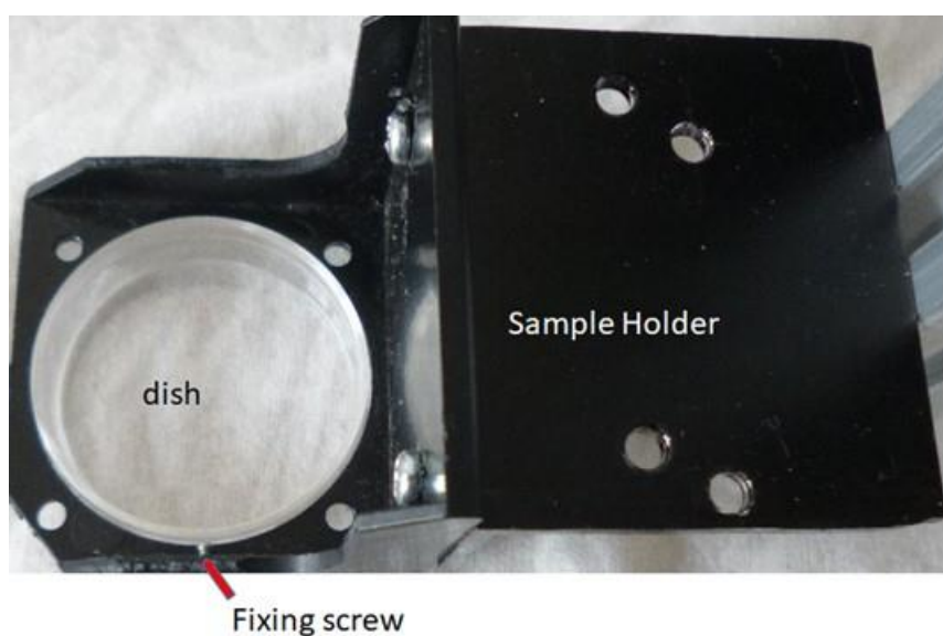
Figure 1-8 placing a dish in the sample holder with a screw so as that the bottom is in close contact with the glass window
