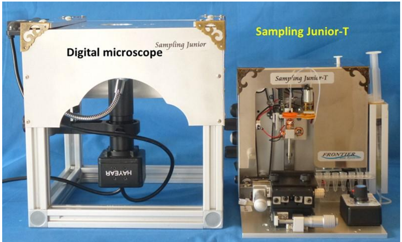
Figure 1-1 Mounting Sampling Junior on a digital microscope
