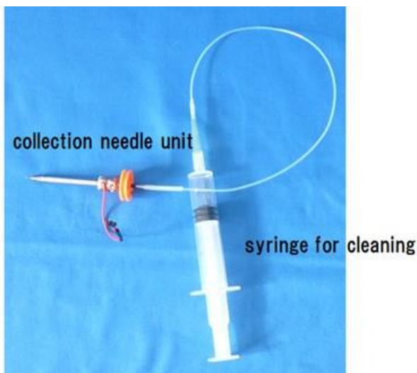
Figure 2-14 Cleaning of a main shaft pipe
