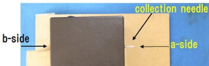
Figure 2-17 Setting for sharpening the edge of a collection needle
