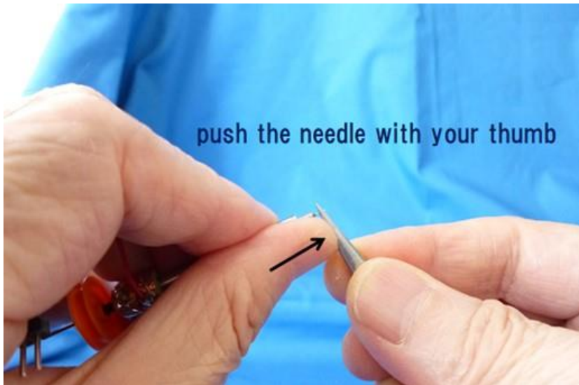
Figure 2-13 the way of taking a collection needle out of the collection needle unit
